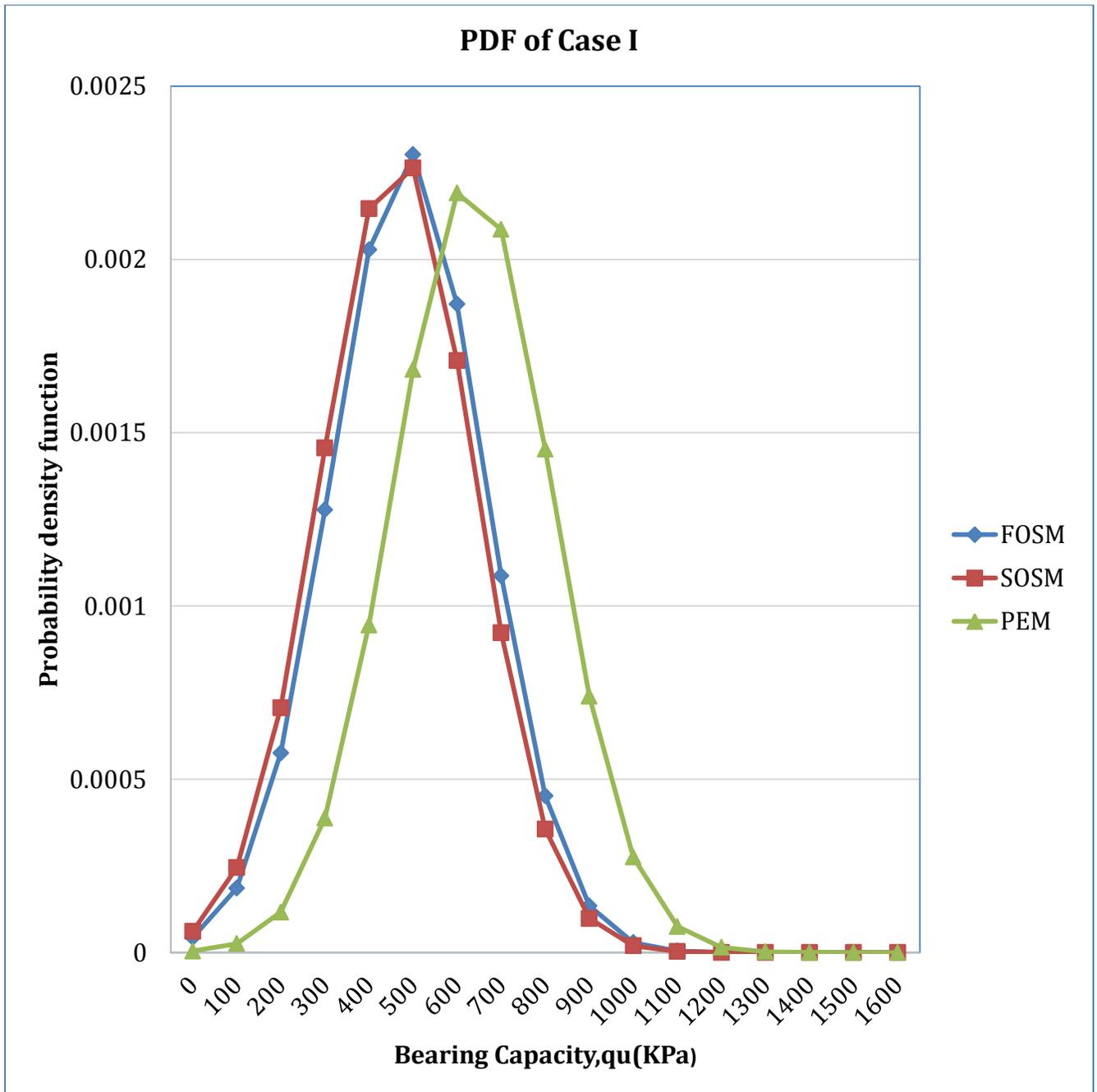
Figure 4-14 : Comparison of results for only friction angle as random variable
