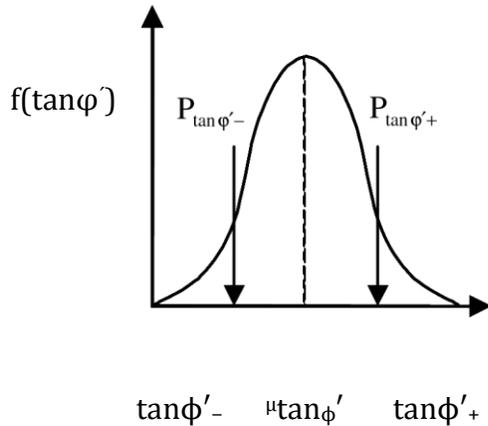
Figure 4-10 : Sampling point locations and weights for  $\tan \phi'$
