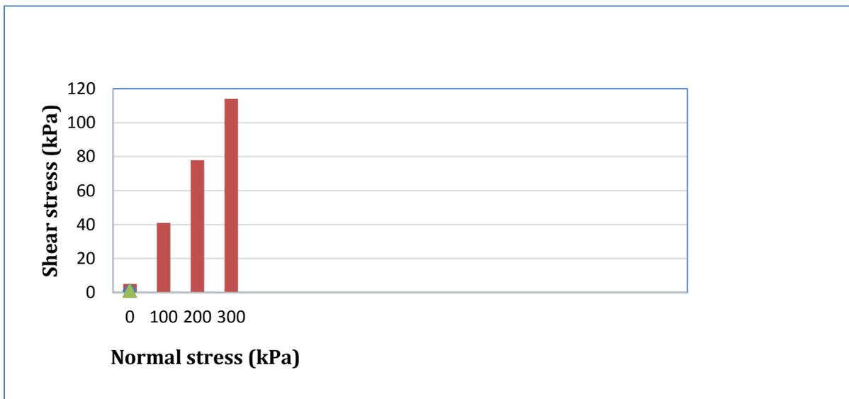
Figure 4-1 : Graphical results of normal stress versus shear stress for sample 1
