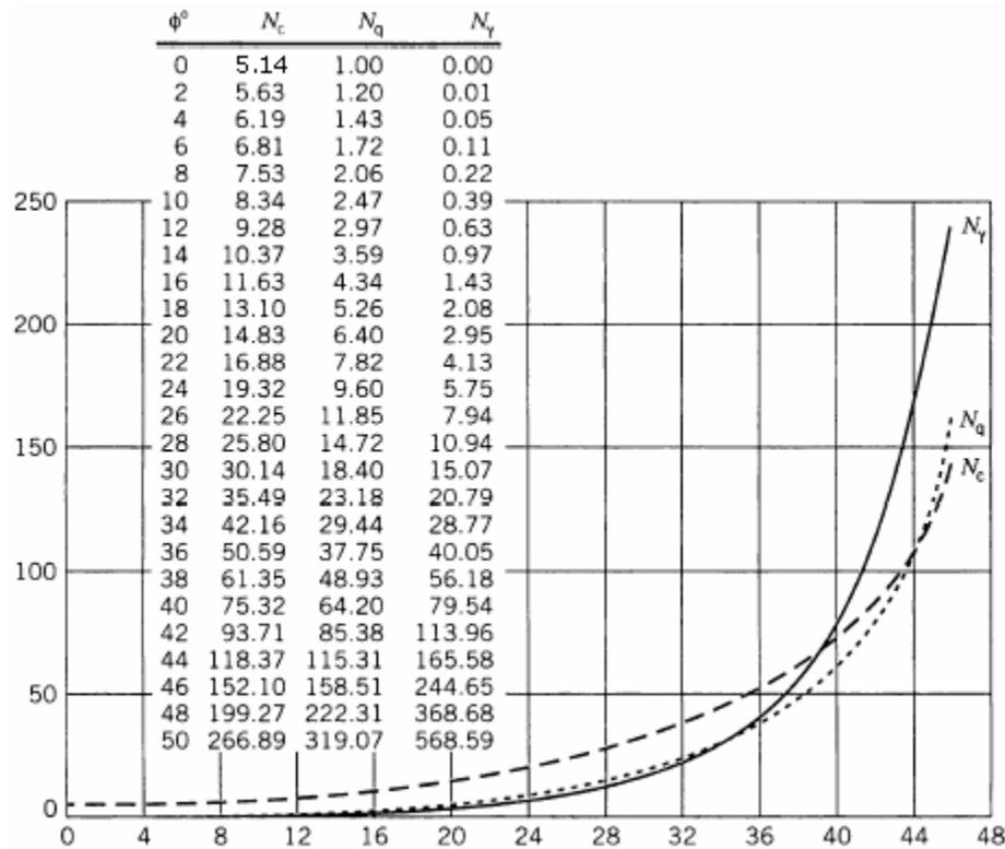
Figure 4-5: Hansen's bearing capacity factors
