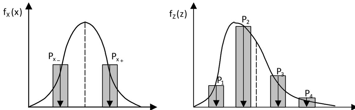
Figure 3-1 : Sampling point locations and weights for a single random variable (a) and for a function depending on two random variables (b)
