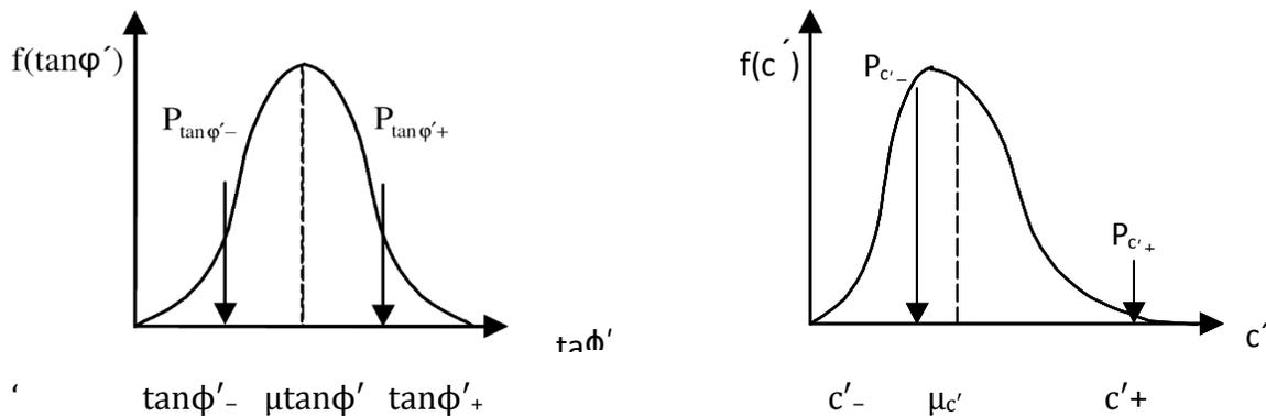
Figure 4-12 : Sampling point locations and weights of the soil parameters  $\tan \phi'$  and  $c'$
