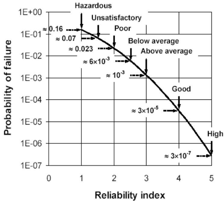
Figure 3-4: Relationship between reliability index ( $\beta$ ) and probability of failure (pf) (US Army Corps of Engineers -1997).
