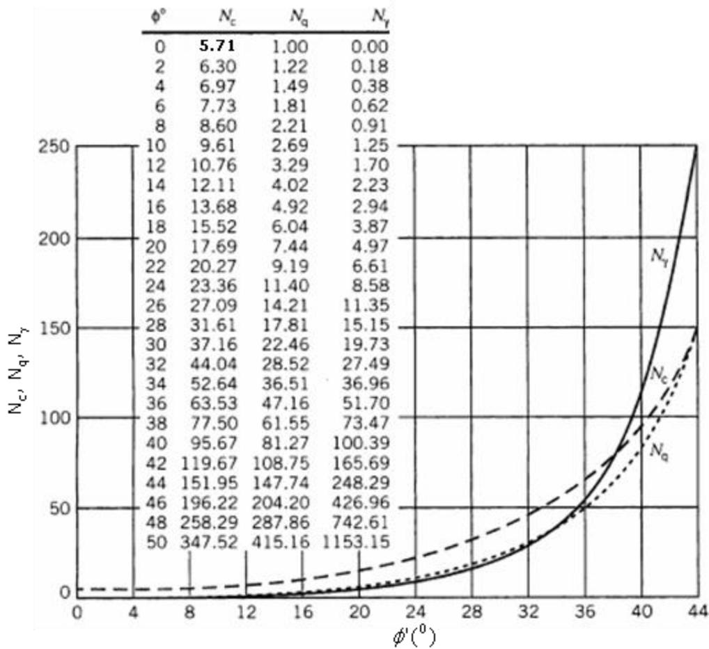
Figure 4-3: Terzaghi's bearing capacity factors
