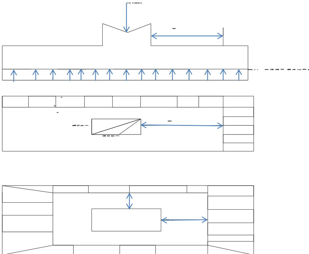
Figure 4-16 : Wide beam and punching shear cross section of footing
