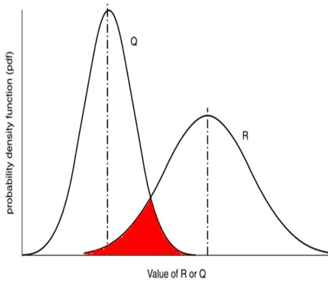
Figure 3-2 : The overlapped area is probability of failure of random variables for Q and R (Subramaniam).
