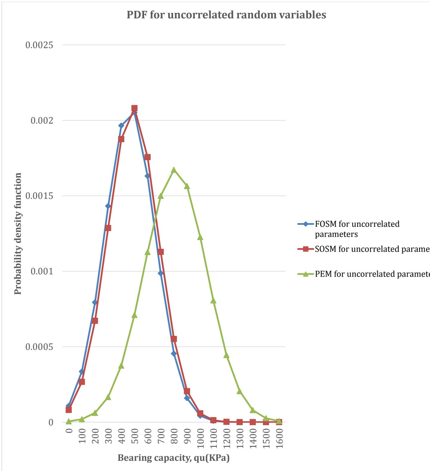
Figure 4-15 : Comparison of results for only friction angle as random variable
