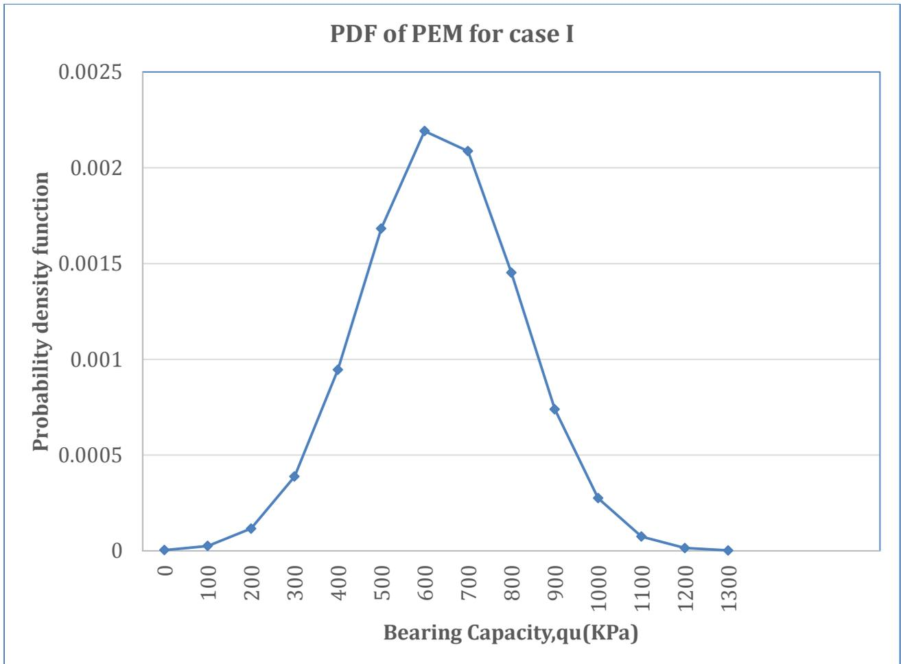
Figure 4-11 : PDF of PEM for only friction angle as random variable
