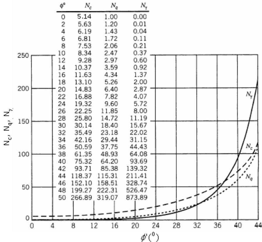
Figure 4-4: Meyerhof's bearing capacity factors
