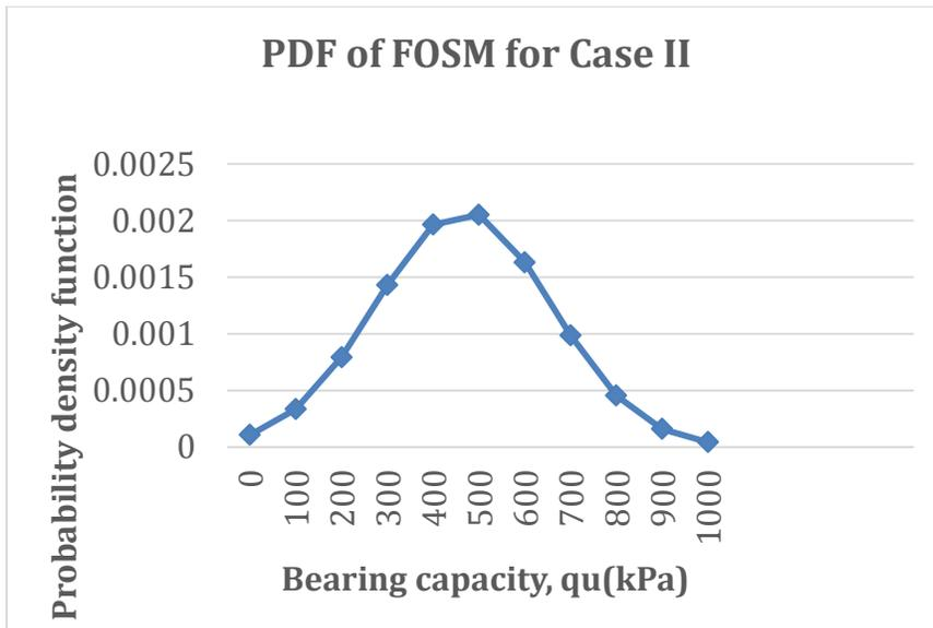
Figure 4-7 : PDF of FOSM for both soil parameters considered as uncorrelated random variables
