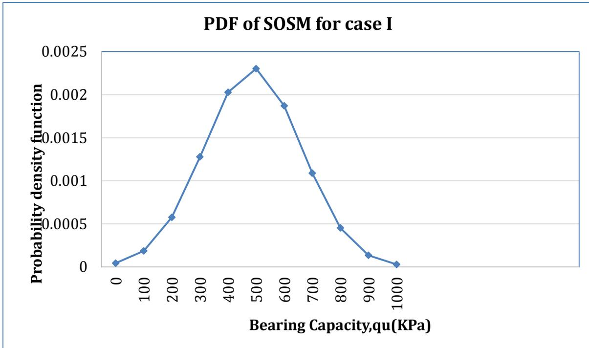
Figure 4-8 : PDF of SOSM for friction angle as random variable
