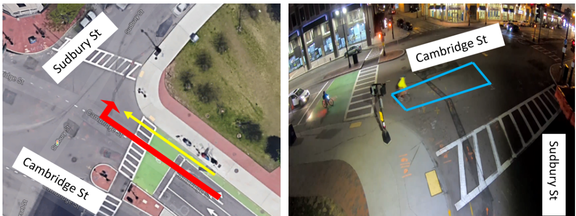
Figure 4.8: Cambridge Street at Sudbury Street (Boston, MA). [Segment: conventional bike lane; Intersection: bike box]
