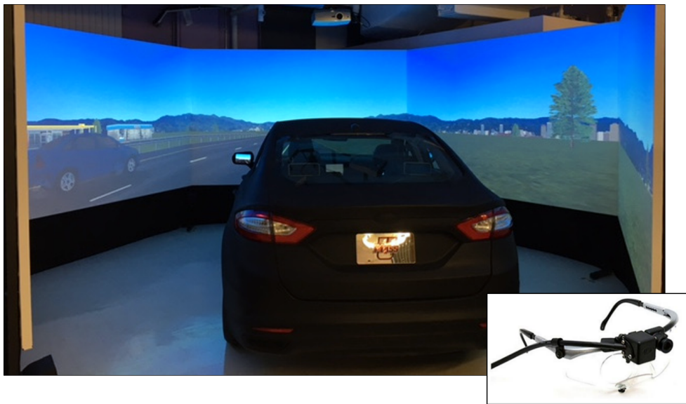
Figure 5.2: University of Massachusetts Amherst Human Performance Lab driving simulator and eye-tracking device
