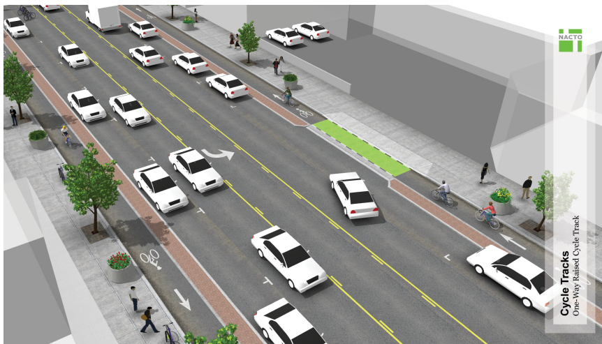
(b) Raised protected bike lane
