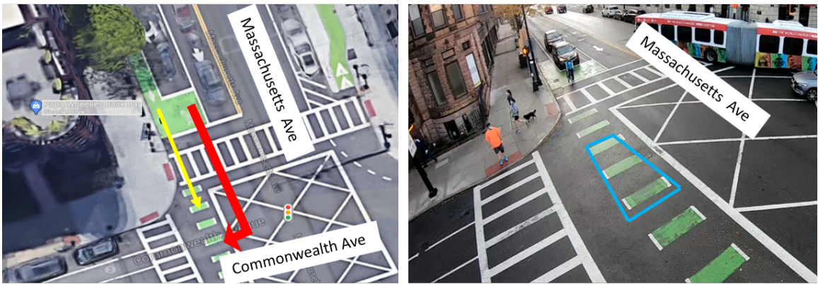
Figure 4.10: Massachusetts Avenue at Commonwealth Avenue (Boston, MA). [Segment: conventional bike lane; Intersection: bike box and crossing markings]
